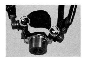
Remove the steering knuckle end bolt by holding its end side with a vise.
