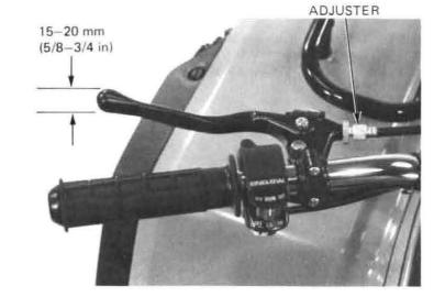
The lever free play can also be adjusted at the lower end of the cable.
