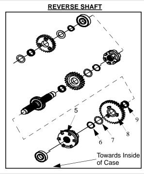
25. Remove the retaining ring (6) and then washer (7), gear (8), and split bearing (9) from the reverse shaft.
