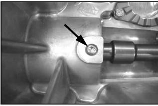
28. Mark the snorkel tube and case with a white pen or marker. This is used to ease reassembly of the gearcase.
