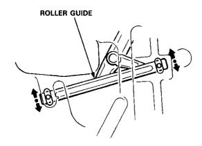
—3 Loosen the locknuts securing the center glass guide, and adjust the glass fore and aft by moving the center glass guide.
