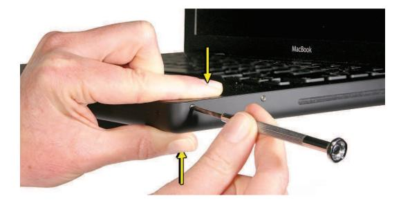
**Replacement Note:** When installing the screws at the rear corners of the bottom case, insert an access card tool between the top case and the display to maintain light pressure as the screws are tightened.
