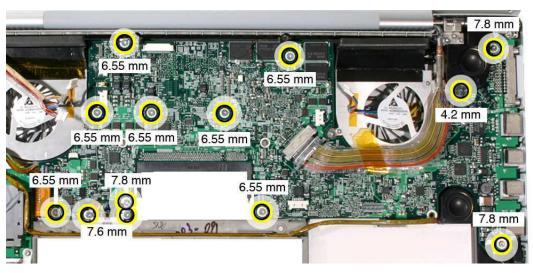
3. Warning: Do NOT allow the logic board to flex at any time. Flexing the board can crack solder joints to components. Give special attention at the narrow neck of the fan cutout.
