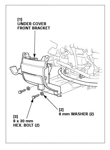
Pass the tube and the wires through the hole in the under cover front bracket.
