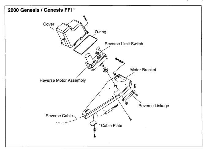
The Genesis watercraft feature an electric reverse gate system designed to make changing direction of travel easier for the operator. A simulated "neutral" gear is possible by positioning the reverse gate half way down. Engine power is limited for safety when the reverse gate is not in the full up or forward position.
